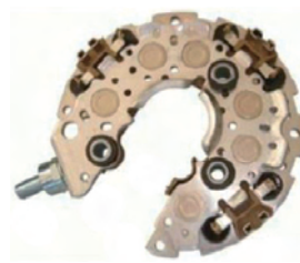
31-82055 Rectifier 117 mm OD M8x1.25 Side Post 120 Amp, 7-50 A Diodes
